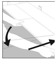
Step 4: Lock long edge of plank by inserting tongue into groove at an angle and drop in place. Slide plank toward end of previously installed plank until the tongue just touches the groove.
