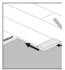
Step 7: Tap end of plank with hammer and tapping block to lock ends of planks together. Remove bridge and continue towards wall until installing the final plank in the row. BE SURE TO TAP ON EDGE OF RIGID SO AS NOT TO DAMAGE LOCKING PROFILE.
