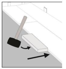
Step 5: IMPORTANT! Use hammer and tapping block to tap long edge of plank to ensure a tight fit. ANY GAPPING CAN COMPROMISE THE LOCKING SYSTEM!
